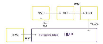
• using NMS only for discovery, where the NMS is used to find out to which OLT the ONT has been plugged in and then UMP changes configuration on the OLT directly. This is the best solution for multi-vendor infrastructures when the service providers want to make their work easier by having a single workflow for all vendor devices;
