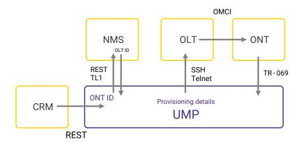
bypassing NMS entirely, where UMP auto-discovers newly connected ONTs across all OLTs. This becomes a must at scale, where the NMS may turn out to be insufficient for handling large numbers of devices, either due to performance issues or missing API integrations that prevent automation.
